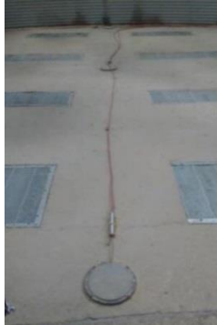
Fig. 3. Placement of sensors for measuring pressure on the silo floor
