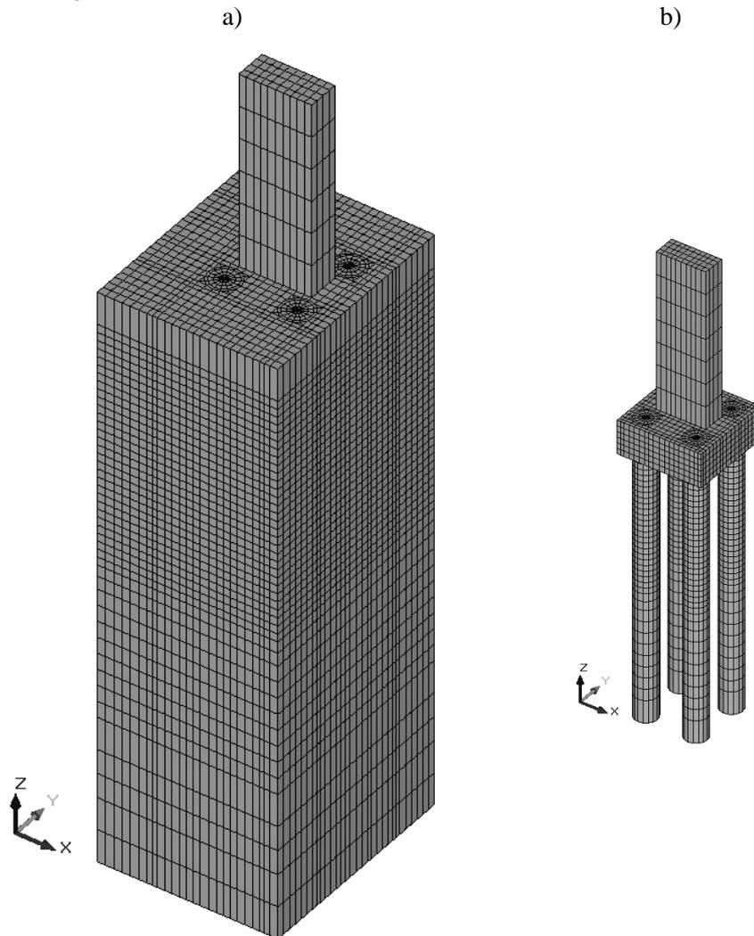
Fig. 2. FE-model and calculation scheme of the pile foundation:
