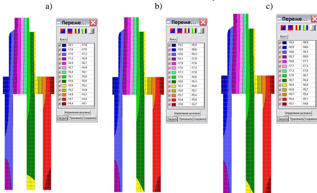
Fig. 4. Isolines and isofields of vertical displacements in a fragment of the abutment model:
