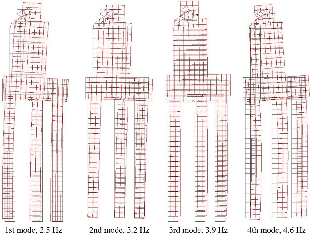
Fig. 5. Modes and frequencies of natural vibrations of an abutment
