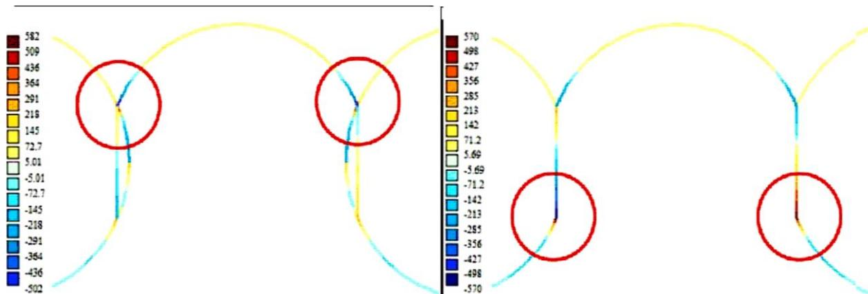
Fig. 10. Mosaic of normal forces values in lining and columns of the station at the sixth (left) and seventh (right) stages of construction
