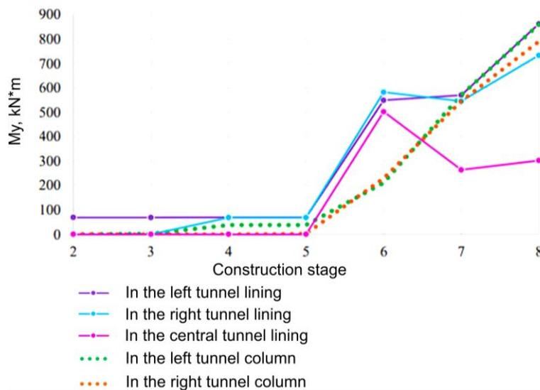
Fig. 13. Graph of changes in the largest bending moments in linings and columns
