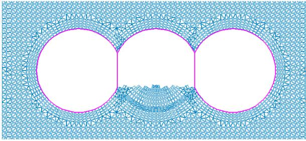
Fig. 6. Finite element model for stage 7
