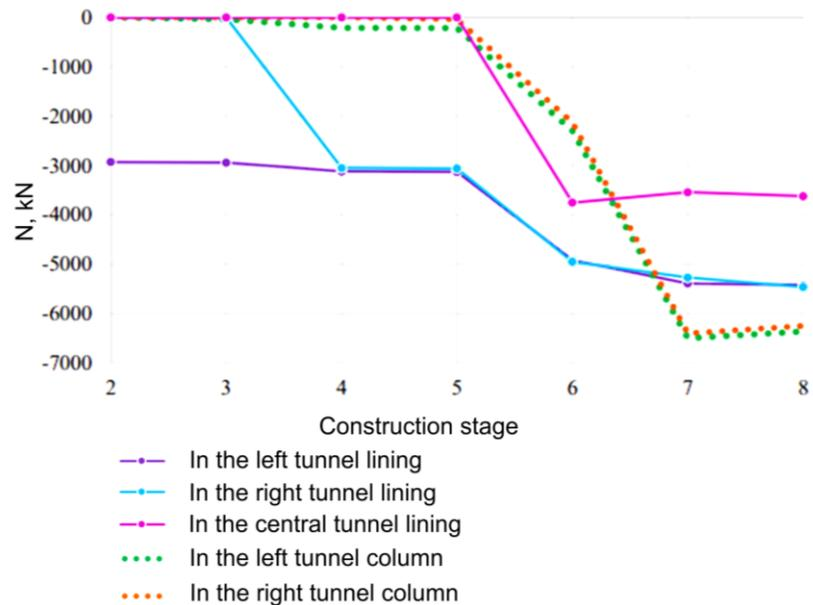
Fig. 12. Graph of changes in the largest normal forces in linings and columns
