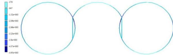
Fig. 8. Force isofields in the lining (stage 6)
