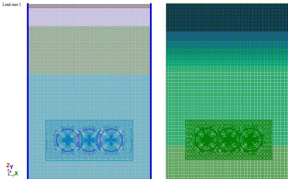
Fig. 2. Finite element model of a column station and soil massif
